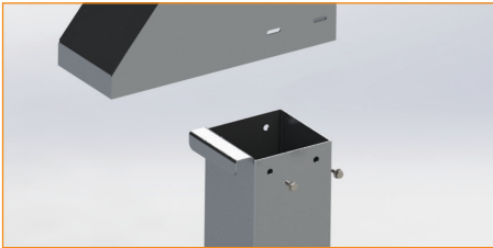
Fixing the cover to the FDD with the supplied screw set
